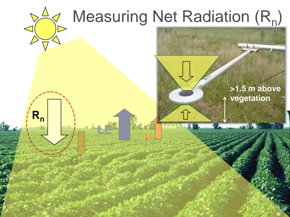
Four component ~ Incoming and Reflected Short-wave and Downward and Upward Long-wave
